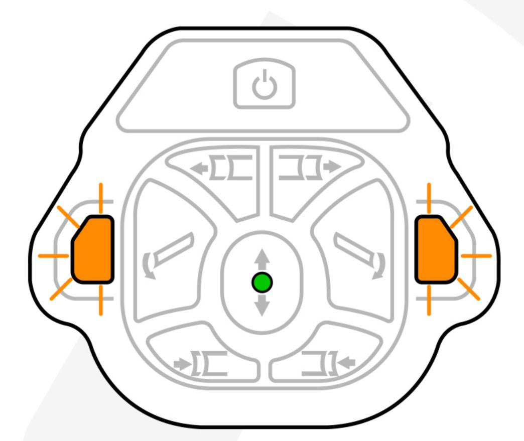
Press the **UP** button to cycle through the flash patterns. Stop on the desired pattern.
