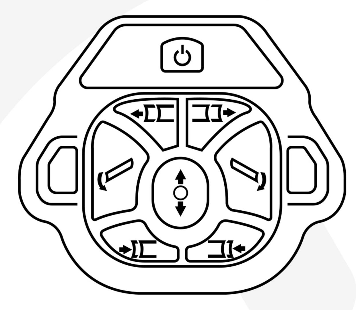
The controller will enter programming mode and the center button will flash Green or Red while in this mode.
